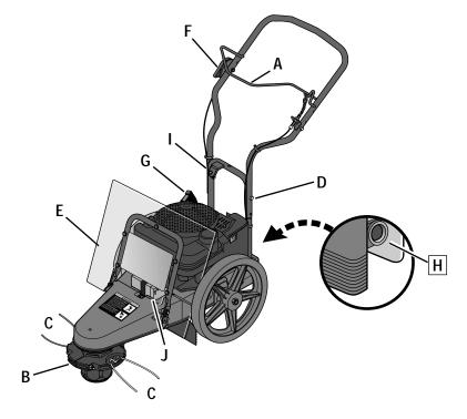
Figure 3-1: Features and controls (electric start model shown).
